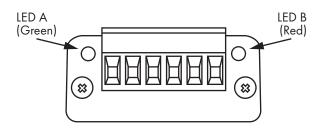
If either LED is not illuminated, the corresponding sensor is not connected correctly or damaged. Check that the connections are made correctly as shown above or replace the sensor.
