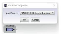
Double clicking on the data input can allow you to select the source as the PT100/PT1000 thermistor input.
