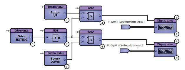
The display Value block should be set to signed and the units applied as Celsius as shown below:
